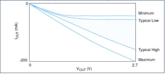
5. The full variation in the ratio of the maximum to minimum pullup and pulldown current will not exceed 1.7, for device drain to source voltages from 0.1 to 1.0.
